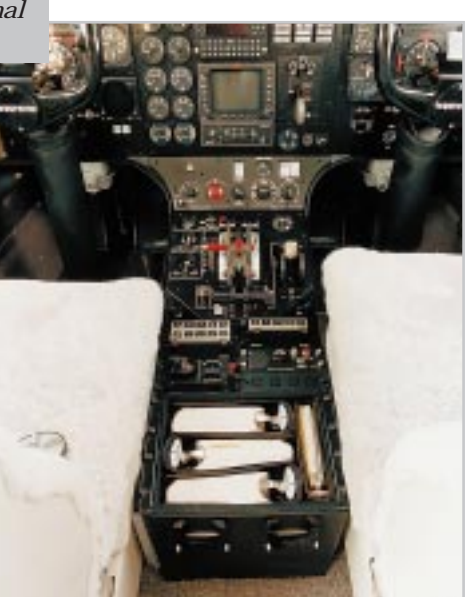
Duncan recently completed a pedestal modification on this Westwind aircraft.
